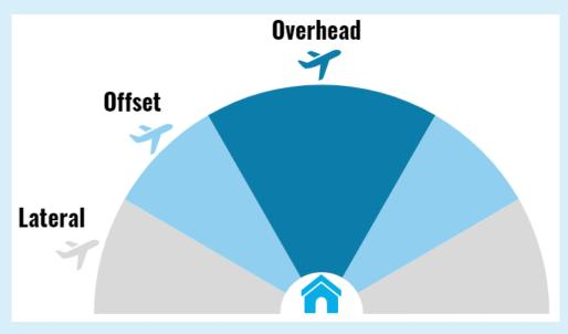
Lateral =  $0^{\circ}$  to  $30^{\circ}$  Offset =  $30^{\circ}$  to  $60^{\circ}$  Overhead =  $60^{\circ}$  to  $90^{\circ}$
